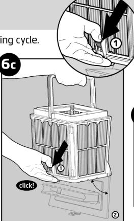
Open the latch to release the bottom lid in order to remove the debris.
