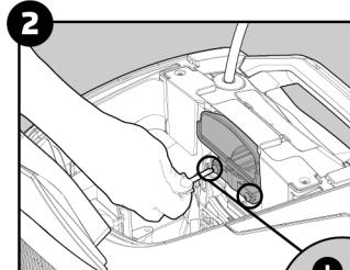
Using a short screwdriver open the 2 screws.
