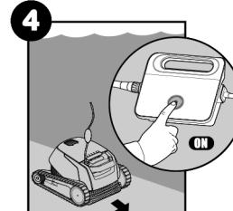
Turn the power supply ON. the pool cleaner will now operate until it has reached the end of the cleaning cycle.
