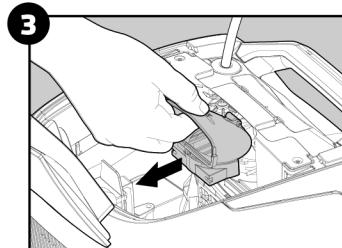
Pull the impeller cover backwards to release it. Clean the debris trapped around the impeller. Assemble the impeller cover.
