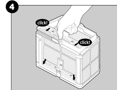
Assemble the filter panels.
